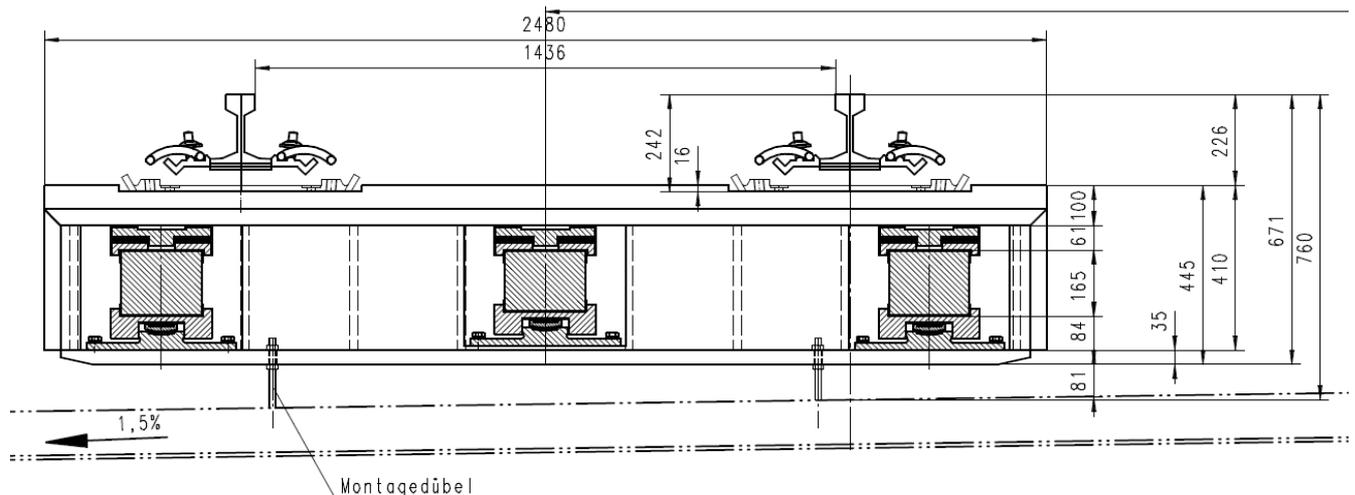
Fig: 1: Section through the MAURER Guided Cross-Tie System Type MS 1
