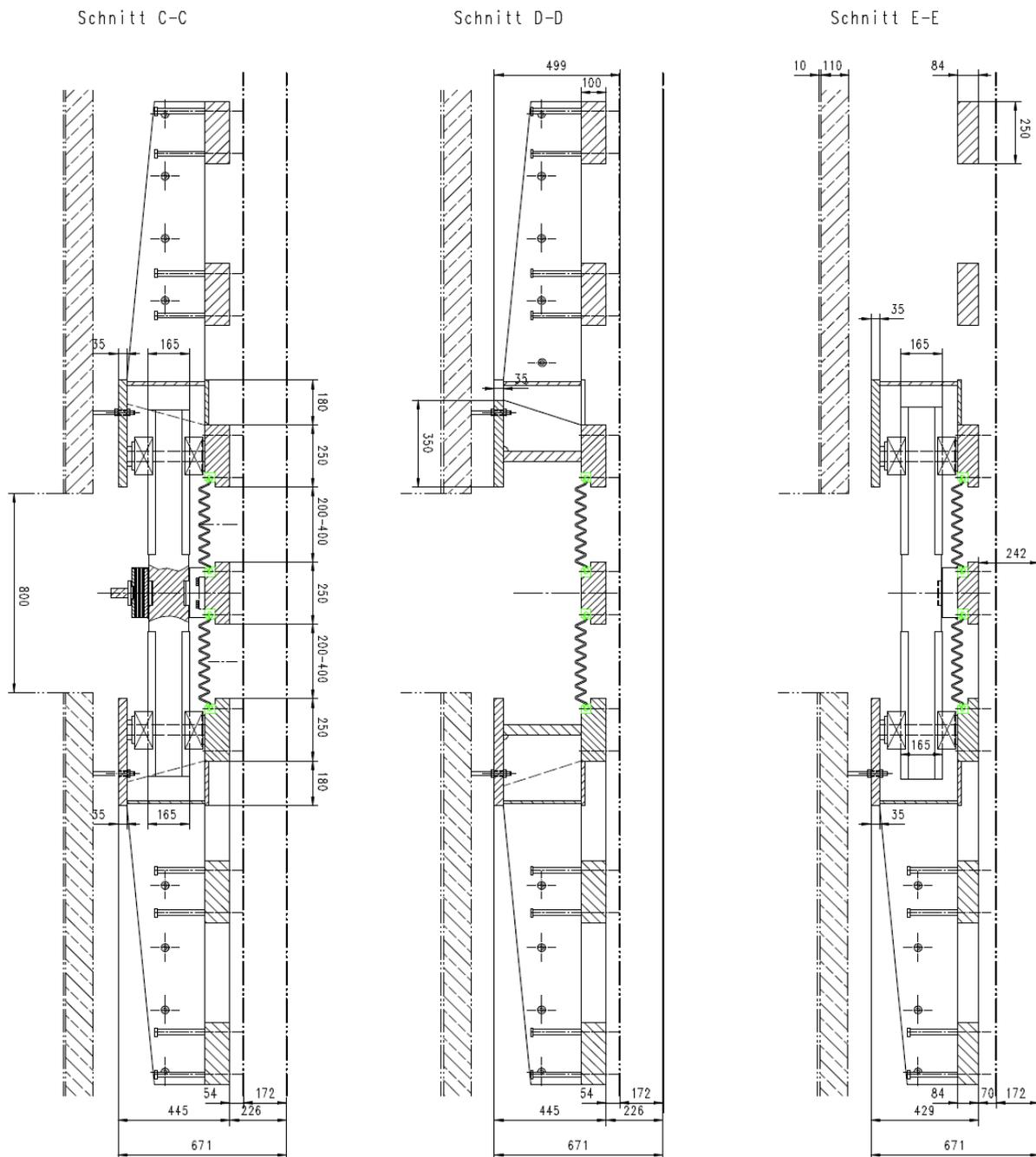
Fig 3: Sections of the MAURER Guided Cross-Tie System MS 1
